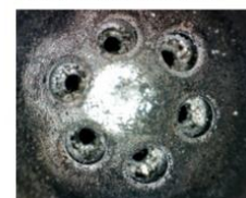
Injector nozzle after cleaning
