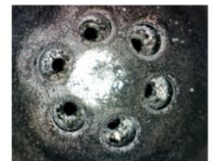
Injector nozzle after cleaning
