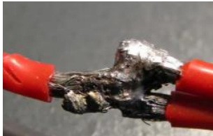
10. Make sure the tin has completely flowed through
