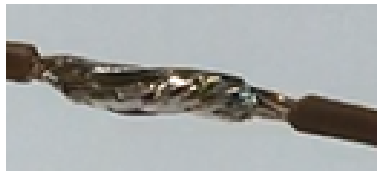
10. Make sure the tin has completely flowed through
