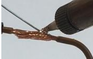
8. Hold the iron tip and solder together on the wire until the solder begins to flow
