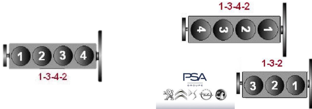
Example of PSA cylinder numbering Beware: First cylinder at gearbox side.
