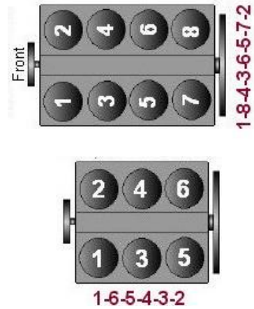
Example of GM cylinder numbering
