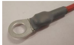
5. Cool down the tubing until the glue is solidified.
