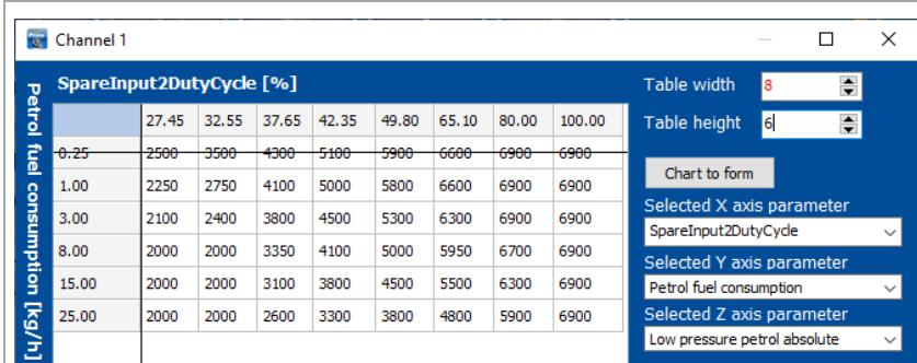
Petrol low pressure Pump duty cycle (%): PWM signal from petrol pump inside petrol tank or signal from petrol pump driver.
