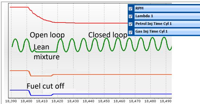
During closed loop the oxygen sensor signals will fluctuate between a minimum and maximum value. Notice these values.
