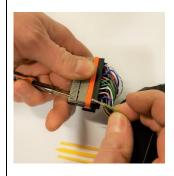
6. Position your tool (very tiny screwdriver or similar) underneath the plastic strip and pull it upwards gently.
