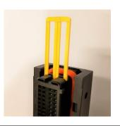
11. After removing or adding a wire, the locking must be returned into its original position.
