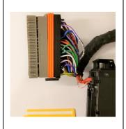
**5.** Put away the middle parts, and locate the pin you need to add or remove.
