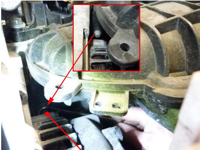
Bolt cannot be removed until complete removal of the manifold.
