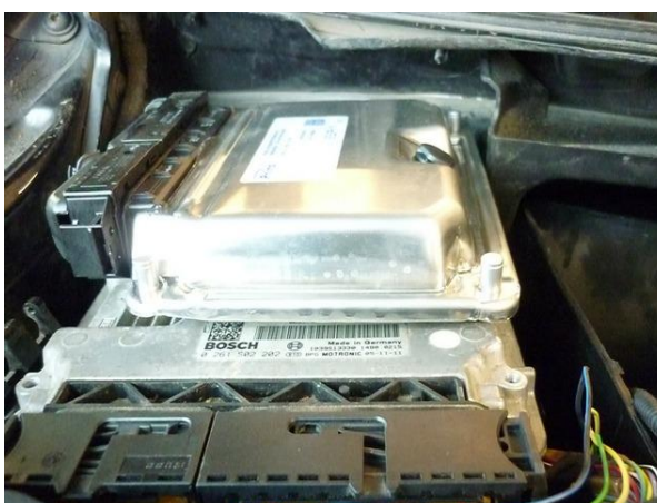
Velcro tape on the AFC &amp; petrol ECU, AFC on the petrol ECU
