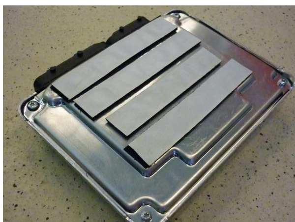
Velcro tape on the AFC &amp; petrol ECU, AFC on the petrol ECU
