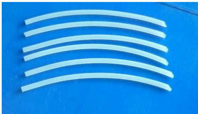
PTFE hose: cut 6x18cm with 45 degree cut (for easy insert)
