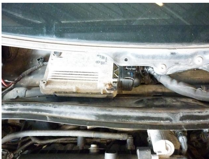
Petrol ECU, remove wipers and panel.
