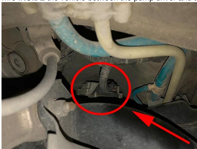
Location of the connector UNDERNEATH the vehicle.
