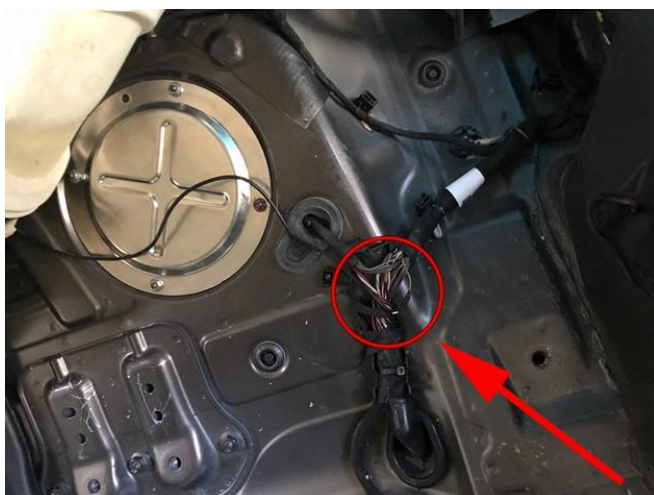
Connect the wire INSIDE the vehicle under the back seat on this location.
