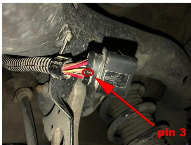
Location of the connector UNDERNEATH the vehicle.
