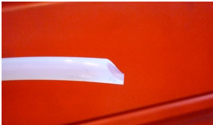
PTFE hose: cut 6x18cm with 45 degree cut (for easy insert)
