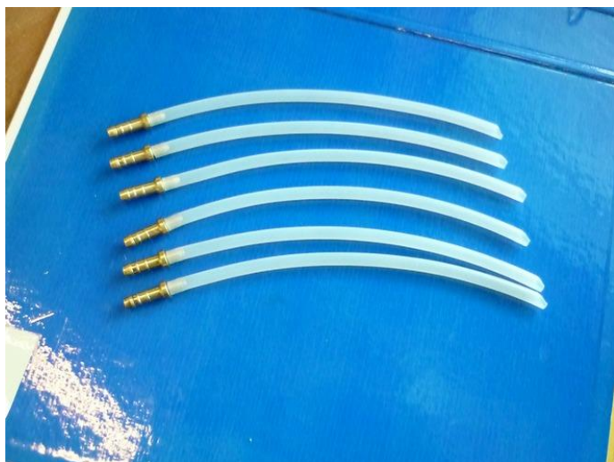
PTFE hose: cut 6x18cm with 45 degree cut (for easy insert)
