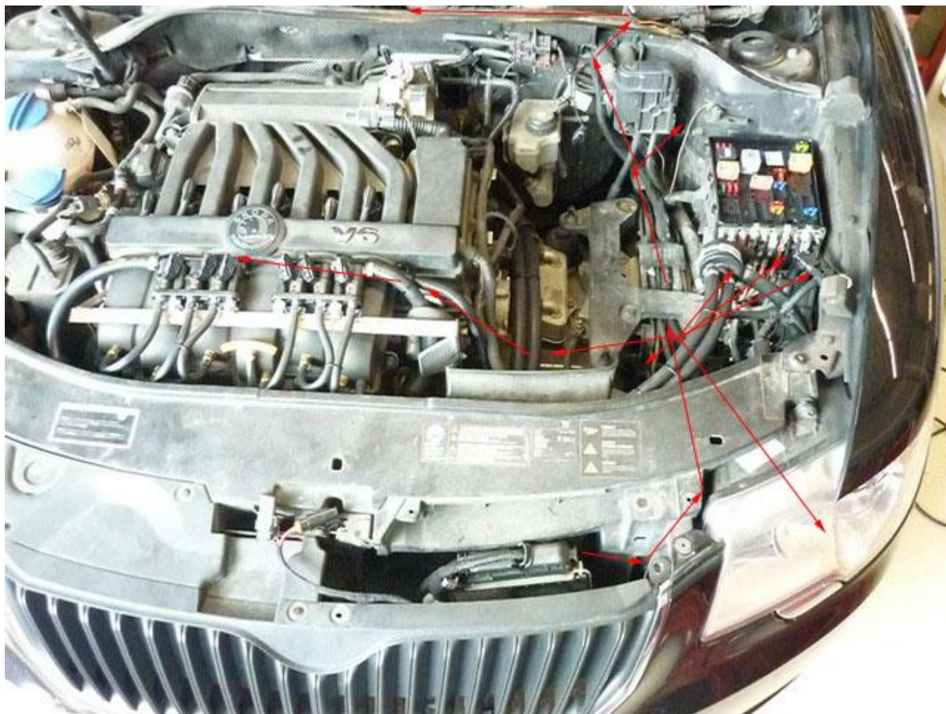
Petrol ECU, remove wipers and panel.
