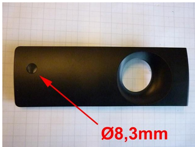
Drill a hole Ø8.3mm for the switch.
