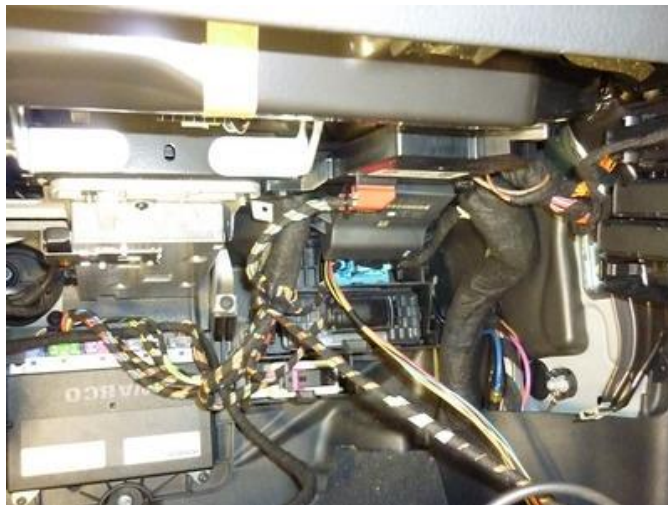
Remove glove compartment for switch wiring.
