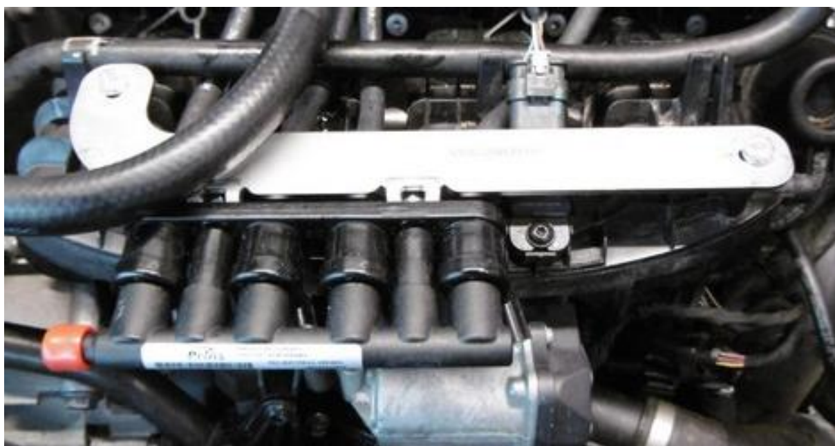
Bracket 001/040230 2x M6 bolt & spring washer
