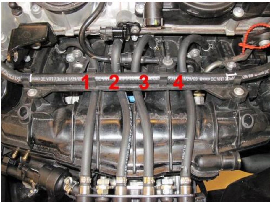
Mount the injector rail with spring washers and nuts. Connect hoses to injector rail.
