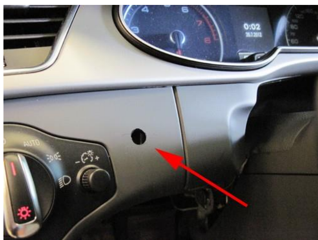
Drill hole Ø8.3mm for mounting switch. Mount switch with the double sided adhesive tape.
