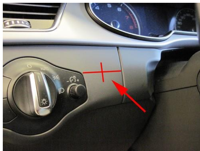
Mark hole for drilling on the right side of the light switch.
