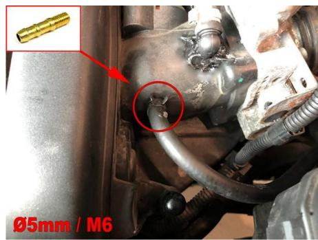
Just behind the throttle body: drill Ø5mm and cut thread M6 and mount the VSI coupling with a locking compound.
