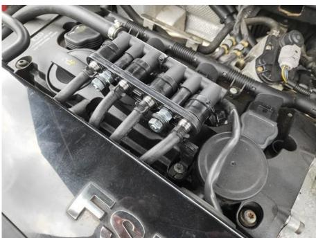
Use and adapt the universal bracket to mount the injector rail.
