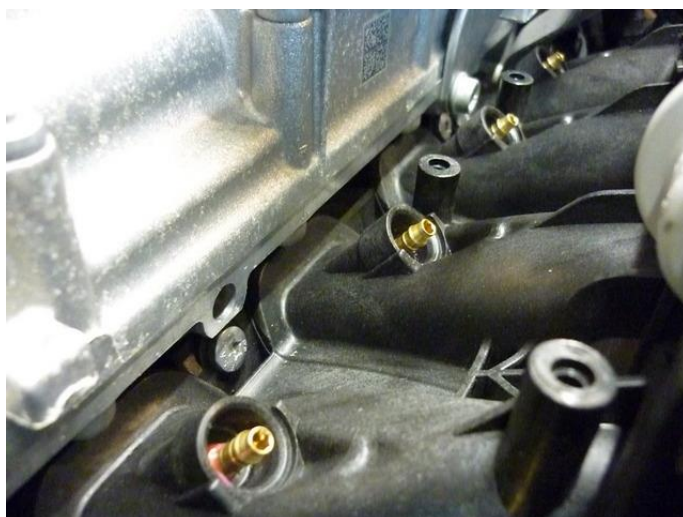
drill Ø5mm – cut M6
