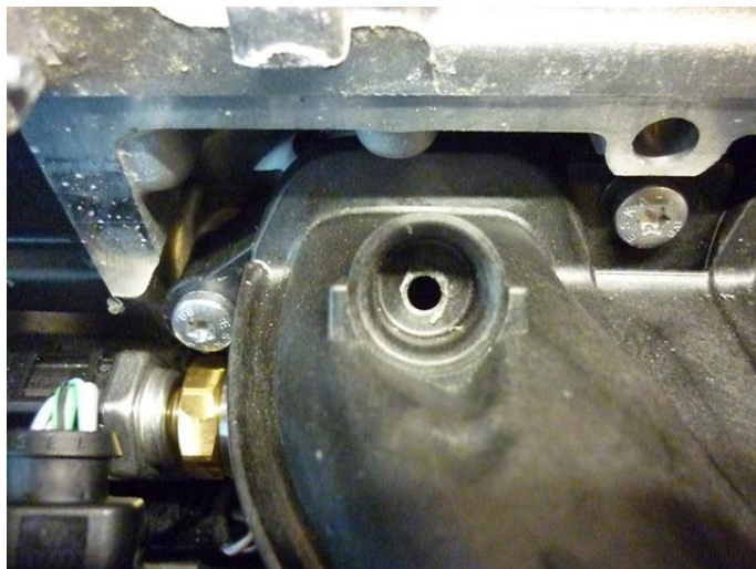
drill Ø5mm – cut M6
