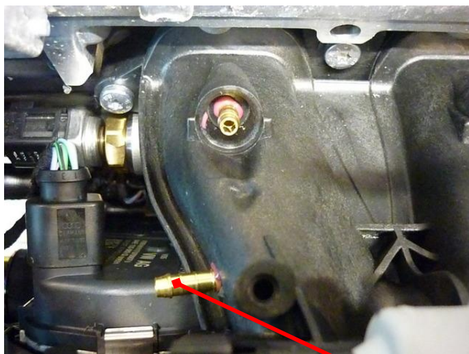
Remove (turn=break) plastic hexagons with 6mm
