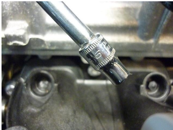
Remove (turn=break) plastic hexagons with 6mm
