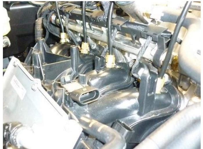
Mount couplings with a locking compound. Mount nylon hoses before mounting the inlet manifold back on the engine
