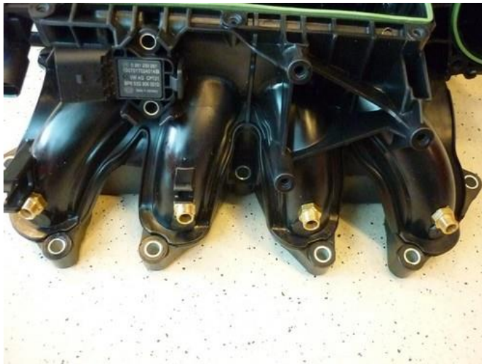
Mount couplings with a locking compound. Mount nylon hoses before mounting the inlet manifold back on the engine
