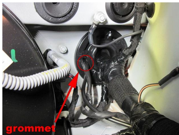
Grommet location for the switch, CAN and fuel gauge reset wires.
