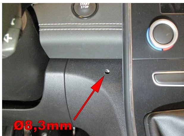
Drill hole Ø8,3mm and mount switch.
