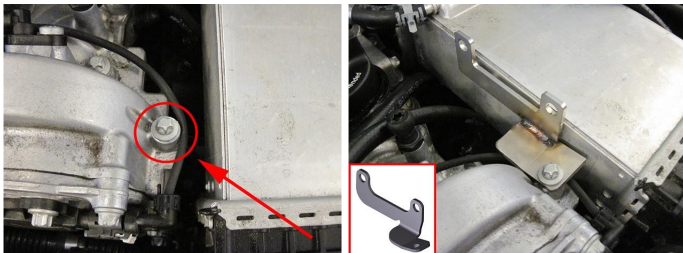
Mount the bracket to the original bolt from the valve-cover.
