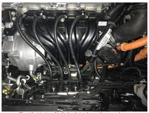
Mount the injector rail to the bracket and mount hoses as shown.
