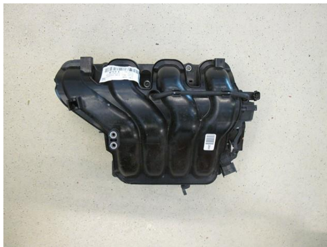
Remove the inlet manifold
