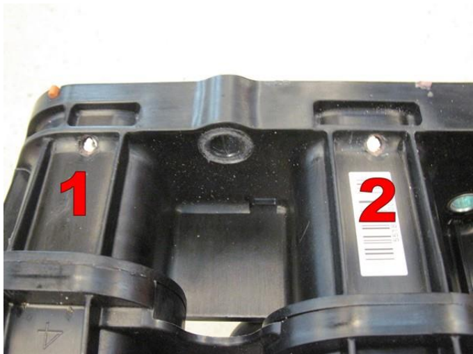
Drill holes 5mm and cut thread M6.
