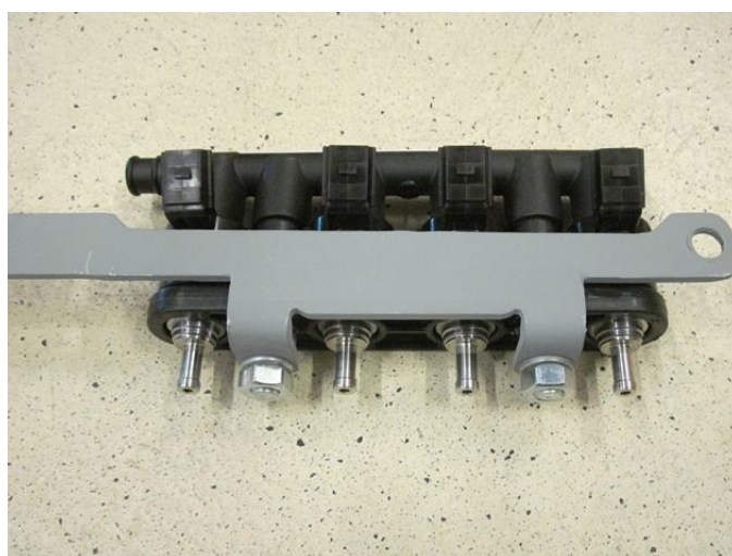
Mount the injector rails to the bracket
