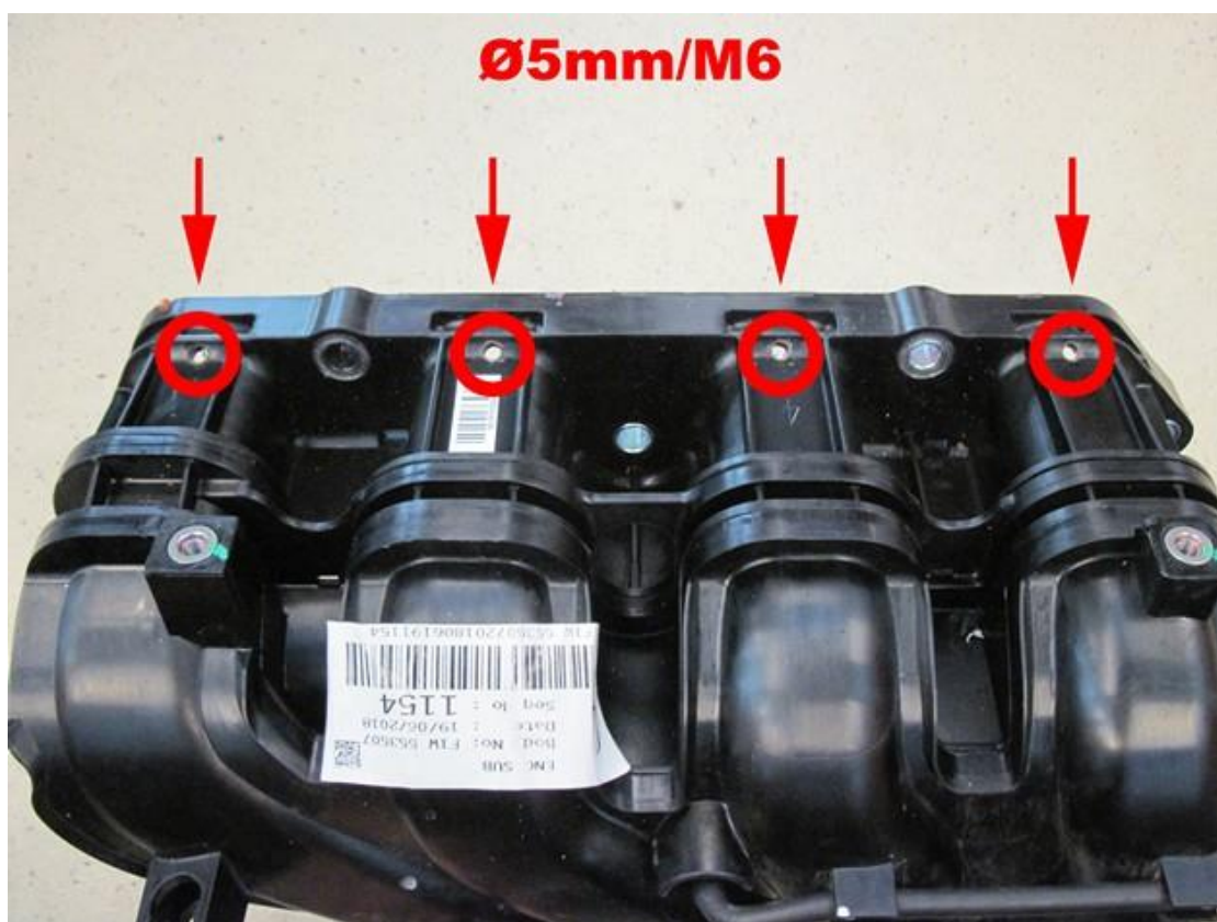
Drill holes 5mm and cut thread M6.
