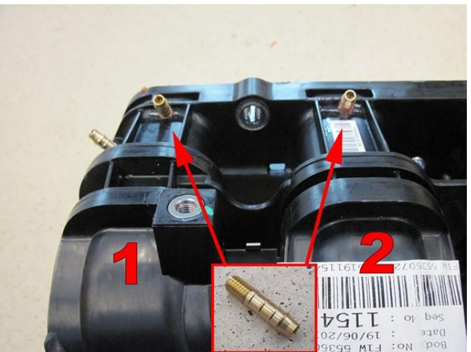
Mount the VSI couplings with a locking compound.
