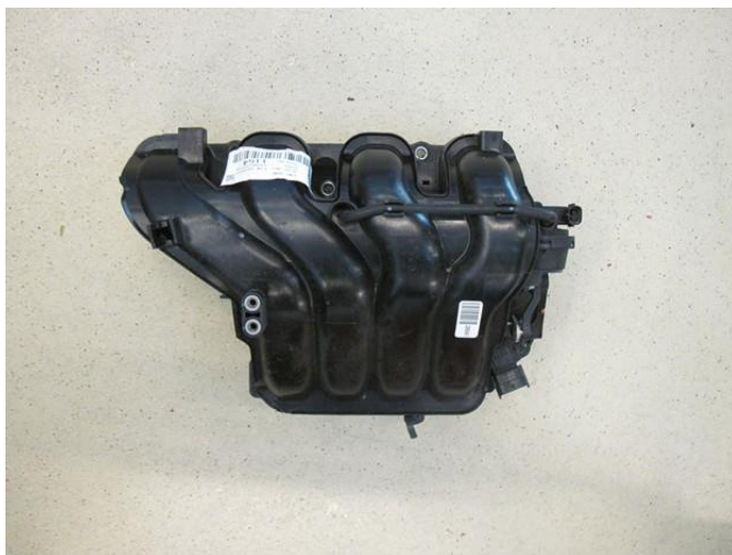
Remove the inlet manifold
