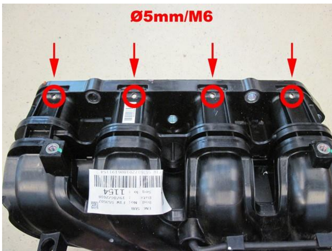
Drill holes 5mm and cut thread M6.
