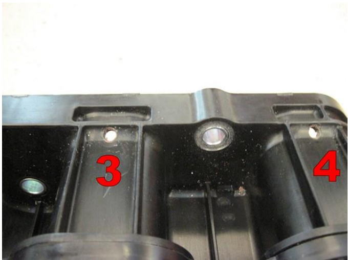
Drill holes 5mm and cut thread M6.
