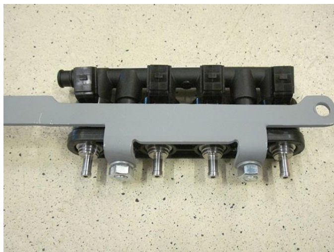
Mount the injector rails to the bracket
