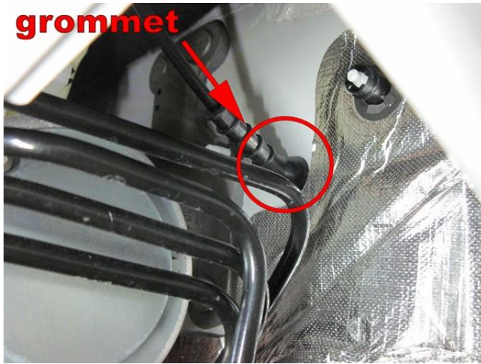
Grommet to use for wiring transit to the driver room.
