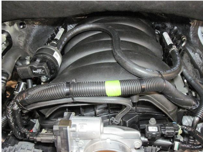
Mount the filter (with sensor) to the bracket on the right bracket and connect the 11mm hoses from filter to both rails.
