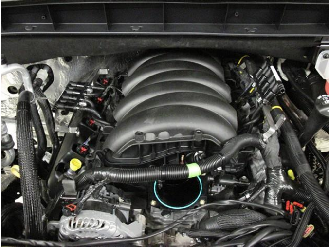
Mount the brackets with rails back to the manifold.
