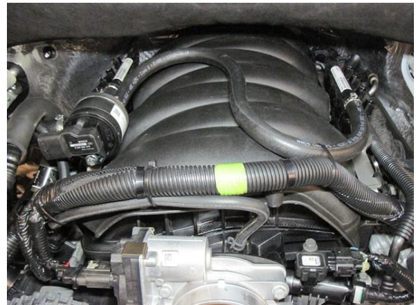
Mount the 16mm hose from the eVP-500 to the filter and mount the 5mm hose to the MAP-coupling.
