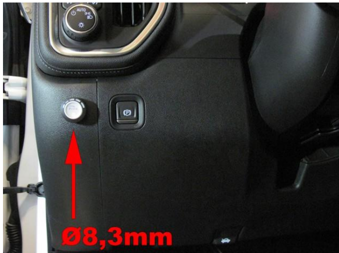
Drill hole Ø8,3mm and mount switch.
