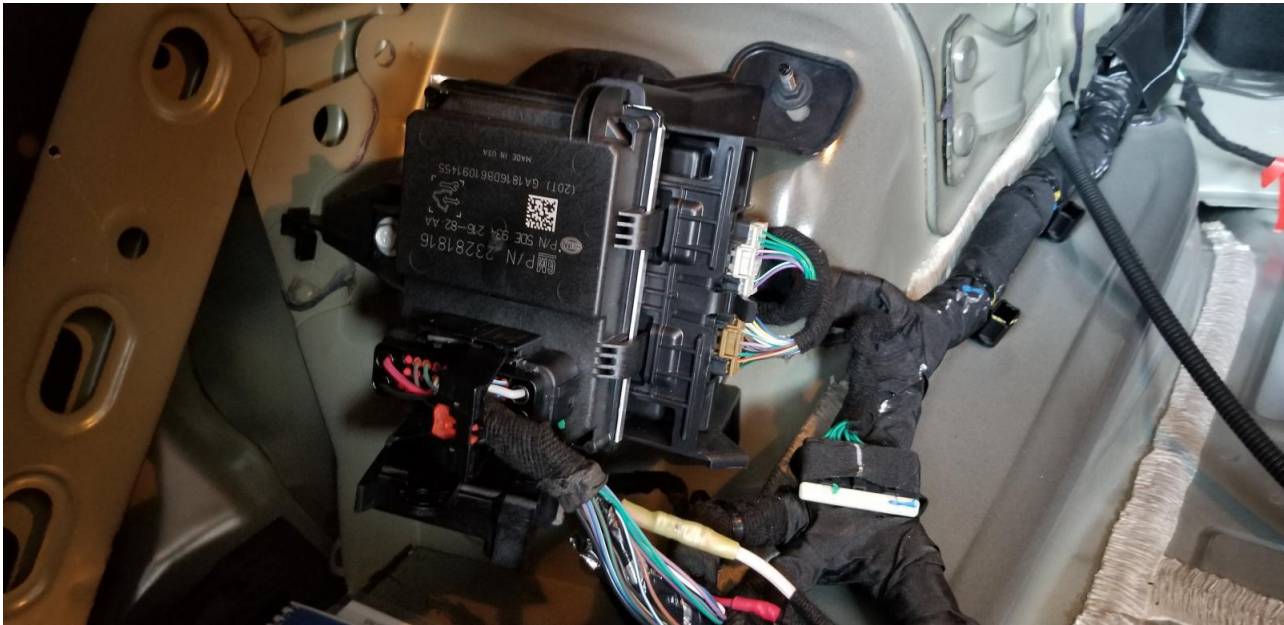
The fuel pump driver control module is located in the trunk on the left side.
