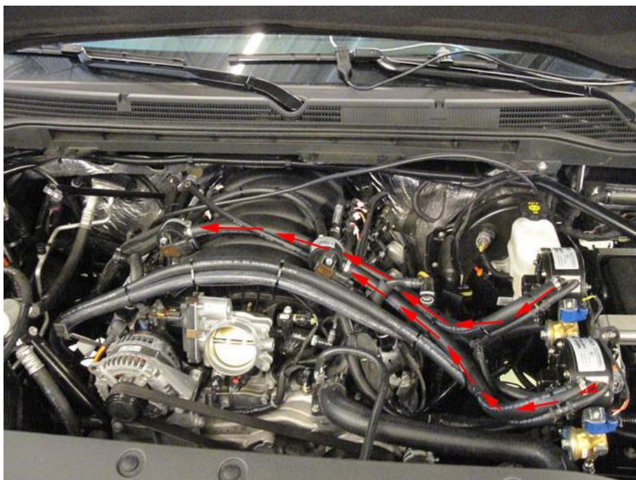
Routing LPG hose from reducers to the filter units
