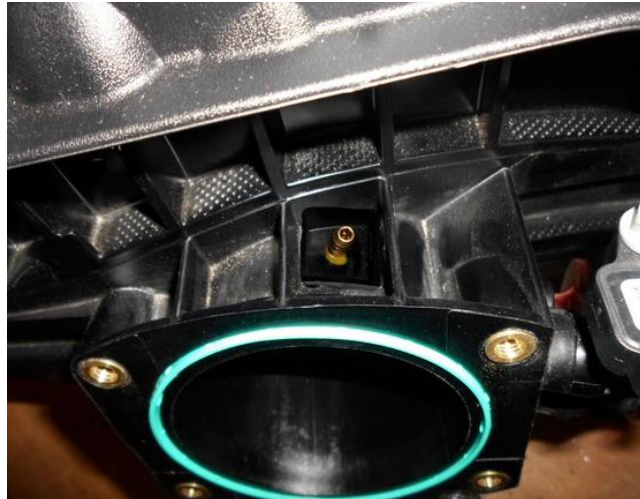
Drill 1 hole of 5mm into the inlet manifold. Cut M6 thread in this hole
