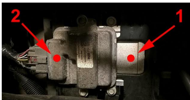
1 = Fuel pump driver control module / 2 = Tow bar control module
