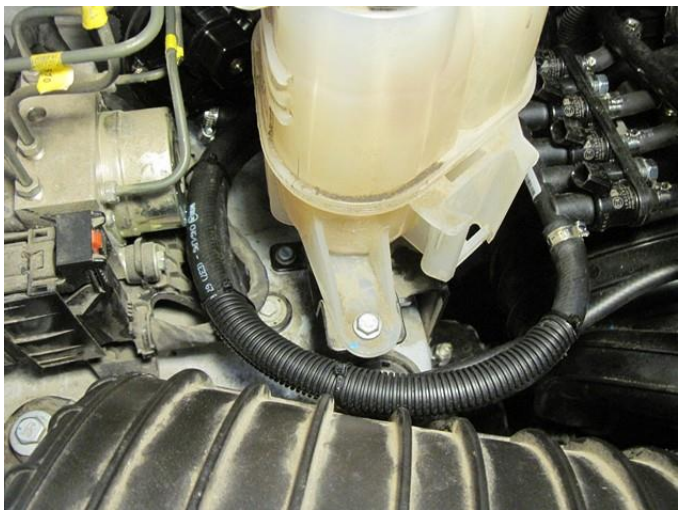
11mm LPG hose routing
