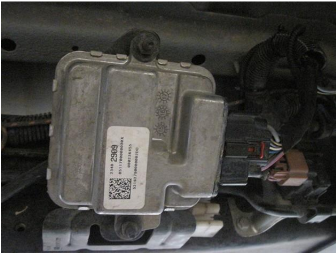
Locate the Fuel Pump Module. At the Chevrolet S10 this is located half-way under the vehicle.
