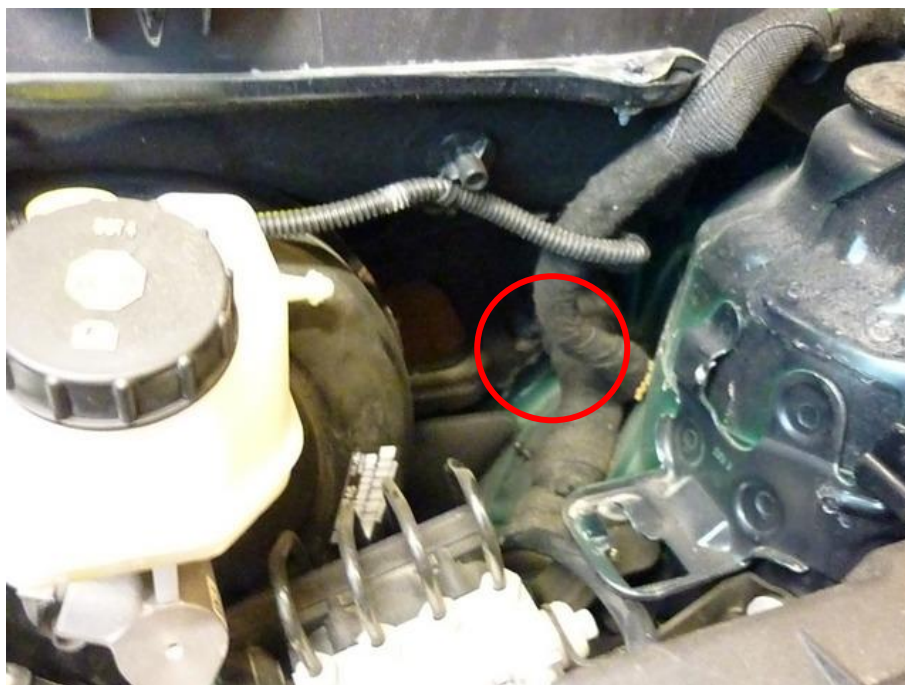
Remove coolant reservoir to reach grommet.
