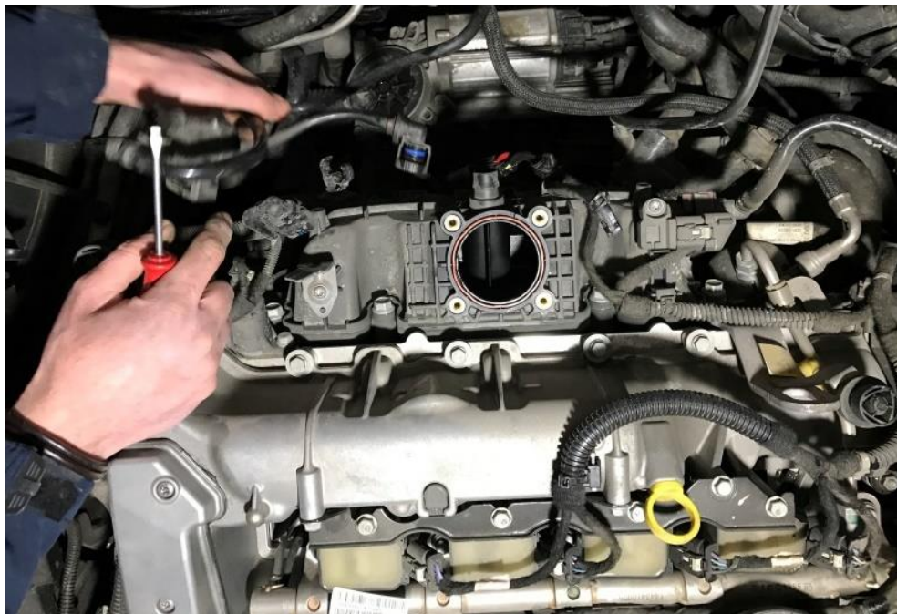
Remove the throttle valve and inlet manifold
