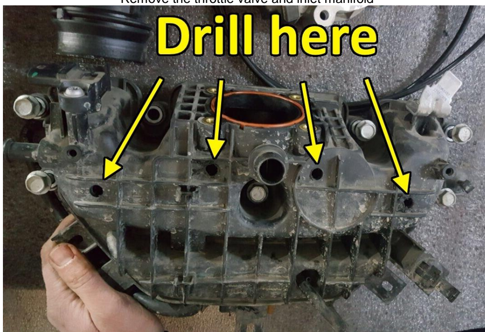
Drill 4 holes of 8,5mm in the inlet manifold. Cut M10x1 thread in these holes.
