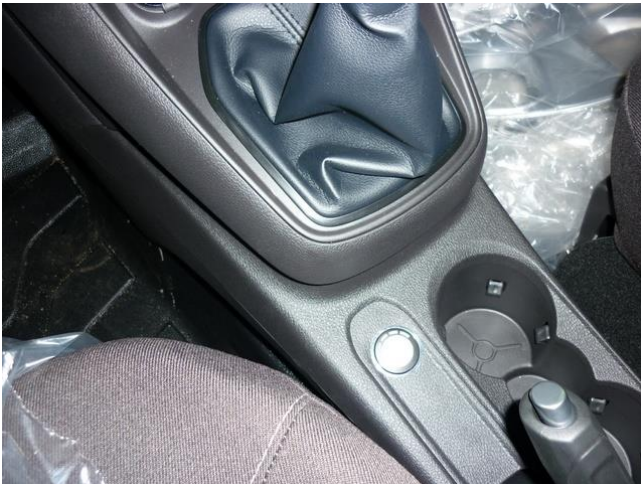
Option 1 (countersunk), drill hole Ø32mm and mount cup.
