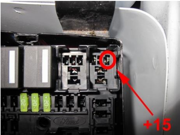
+Ignition in fuse/relay box on left side of engine bay.
