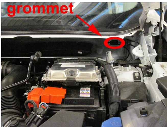
Examples grommet location from Ford Transit Courier 2015 RHD
