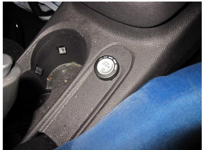
Option 2: on top, drill hole 8.3mm.
