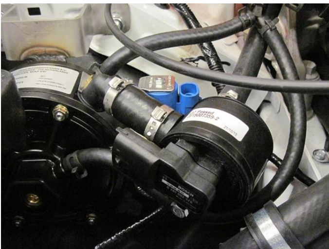
eVP can be mounted on the same location, together with filter.
