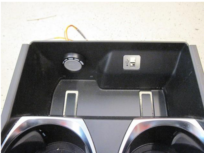
Mount switch and mount the tray back to the vehicle.
