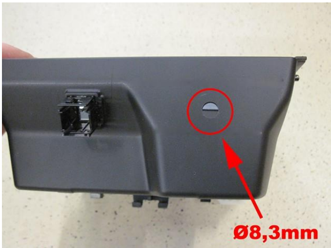
Push the plastic tray to the front and lift out of the vehicle (disconnection wires) . Drill hole Ø8,3mm for the switch.
