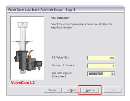
• By clicking the "Next" button, the ValveCare unit will calculate the correct amount of ValveCare fluid (indicated in: injection time per additive dosage).
