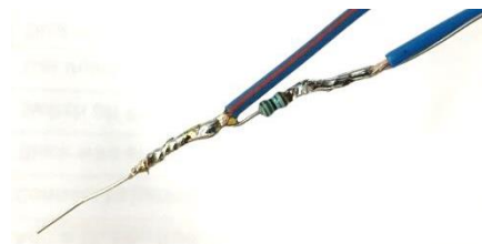
Solder the wires
