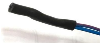
Shrink the sleeve and solder the resistor wires onto the wiring loom
