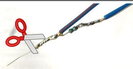
Cut the resistor wires (7mm)
