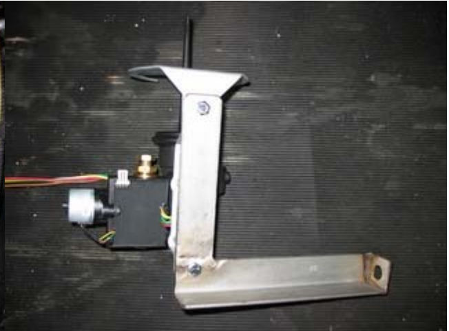
mount the valve care unit onto the bracket
