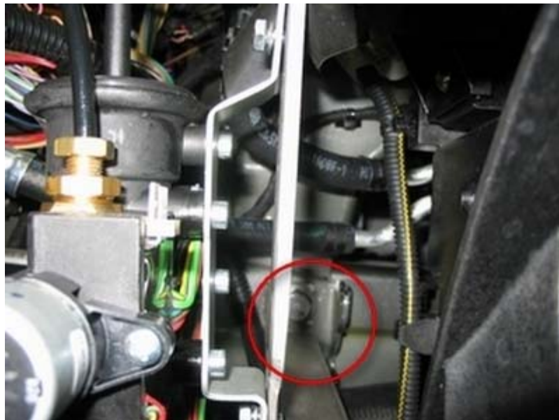
install the unit with the bracket with the removed M10 bolt
