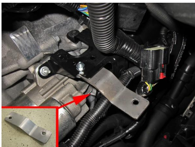
Mount support bracket just above starter. Mount FSU / FRU / Boost pump bracket.
