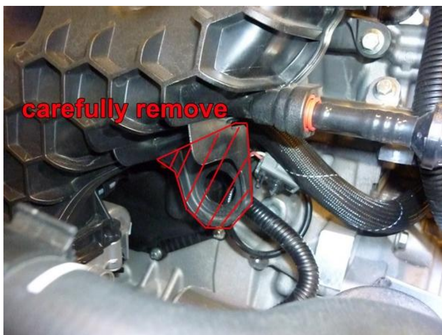
Carefully remove from inlet manifold
