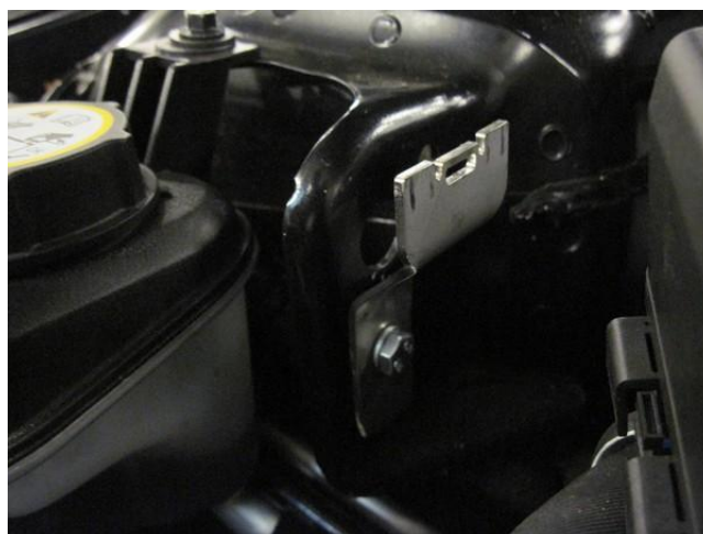
Mount fuse / relay bracket
