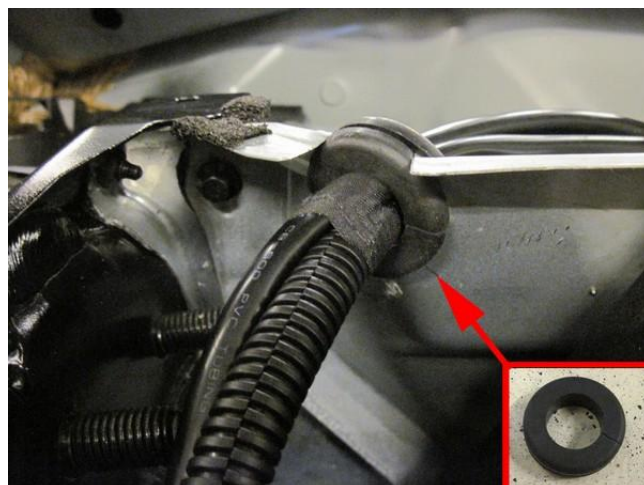
Mount wiring with grommet to vehicle. The same for the wiring transit at the battery box.
