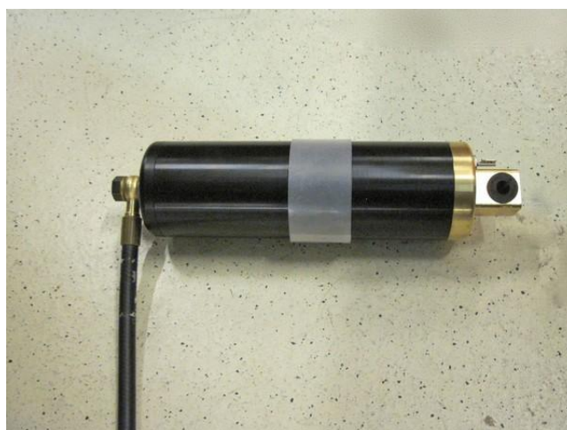
Mount FSU / FRU / Boost pump bracket. Mount boost pump with hose to bracket with clamp & rubber sleeve.
