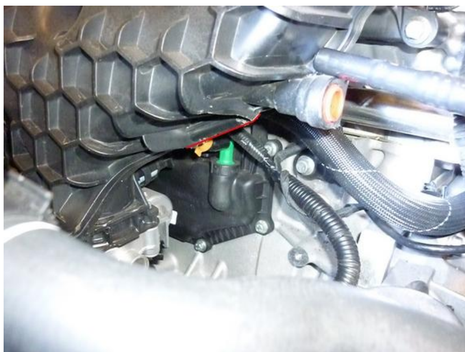
Carefully remove from inlet manifold
