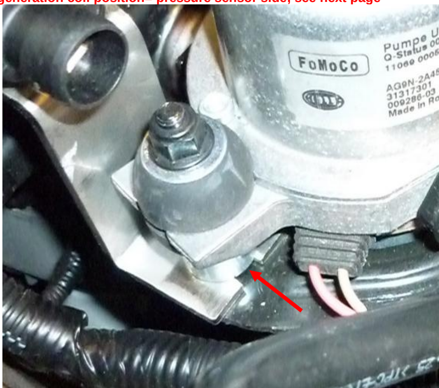
Bracket underneath pump spacer.
