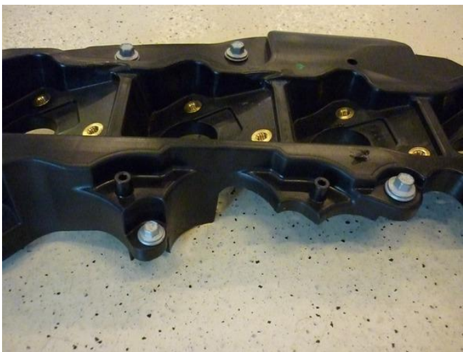
Adapt cover. Remove bolt ( cut away )
