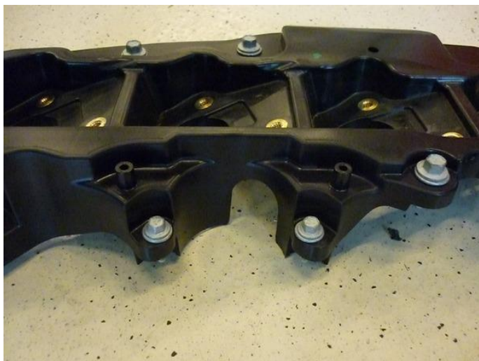
Adapt cover. Remove bolt ( cut away )
