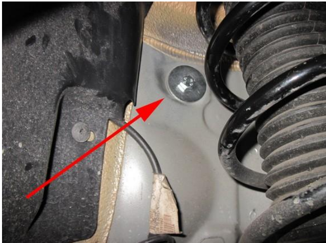
Mount bracket with FSU & FRU to vehicle.
