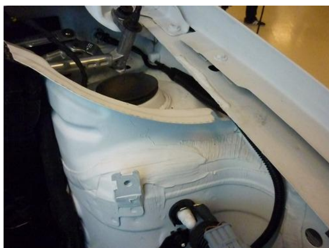
Option 2: Switch wiring next to bonnet release cable ( secure wiring with straps to the cable )
