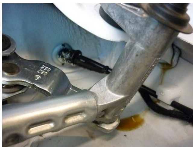
Option 2: Switch wiring next to bonnet release cable ( secure wiring with straps to the cable )
