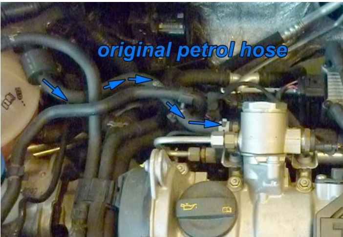
Connect the fuel hose with the XD-5 banjo eye to the inlet of the boost pump.
