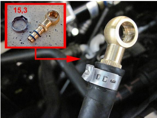
Connect the fuel hose with the XD-5 banjo eye to the inlet of the boost pump.
