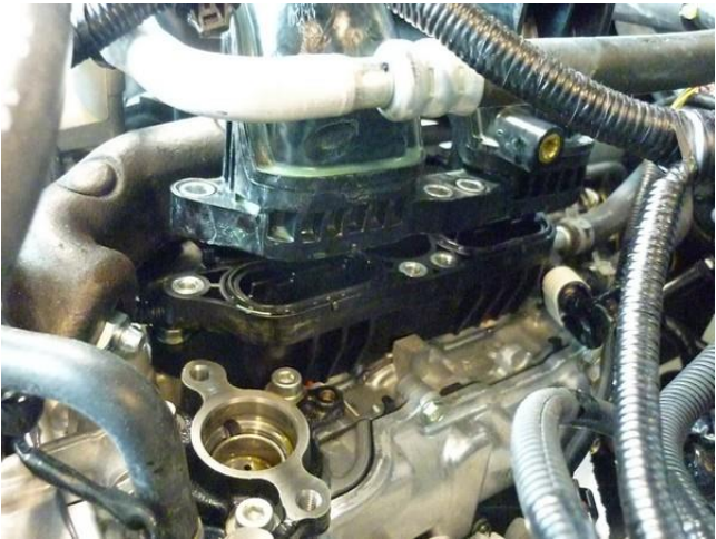
Remove valve housing, left side ( 4 ) for removing the high petrol pressure pump
