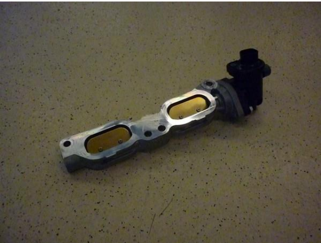
Remove valve housing, left side ( 4 ) for removing the high petrol pressure pump
