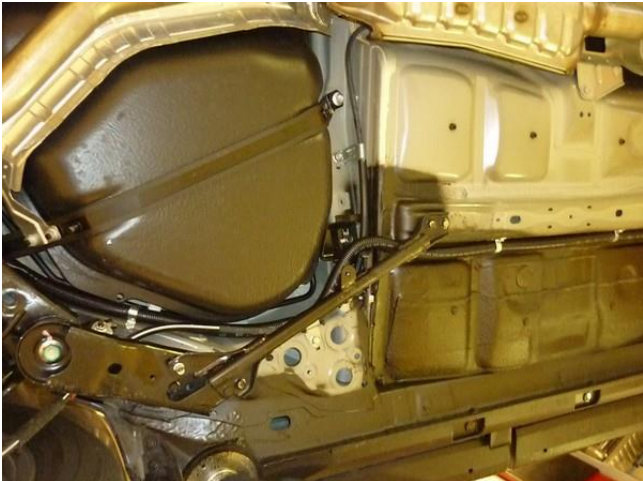
Temporary loosen bolts/nut for fuel lines and wiring
