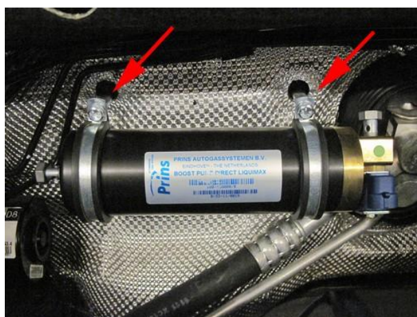
Mount boost pump with clamp, bolts and spring washers to spacers.
