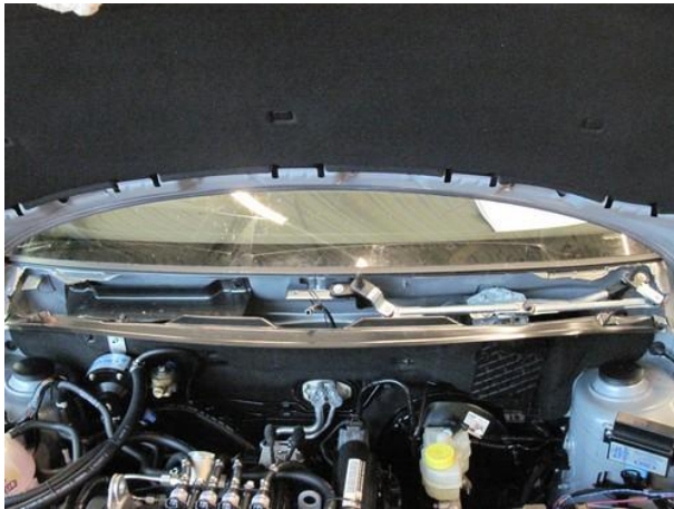
Remove wipers, wiper box cover and wiper motor.
