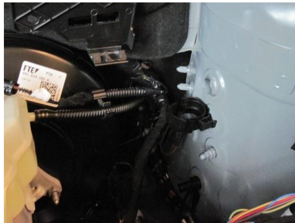
Transit wires from engine room to wiper box through grommet.
