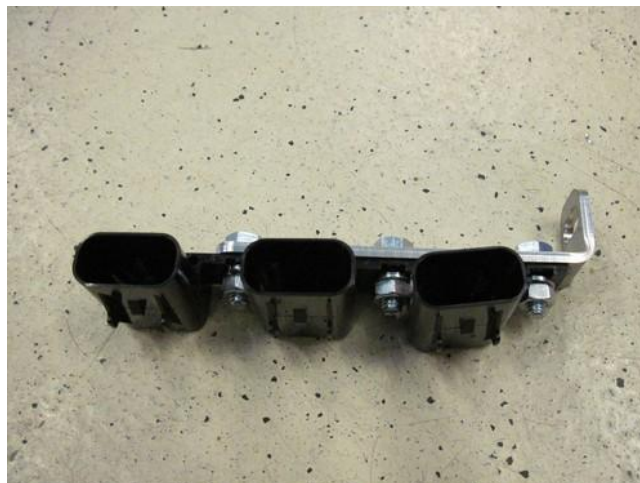
Mount fuse holders to bracket
