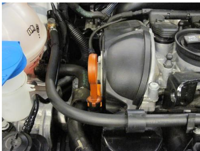
Mount XD-5 eye with clamp to fuel hose. Mount 8mm fuel hose with banjo bolt to Fuel Quick Connector.
