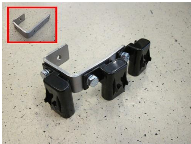
Mount fuse holders with M6 bolts and spring washers to bracket. Mount brackets with fuses & diagnostic connector to original bracket (see picture) with M6 bolt and spring washer.
