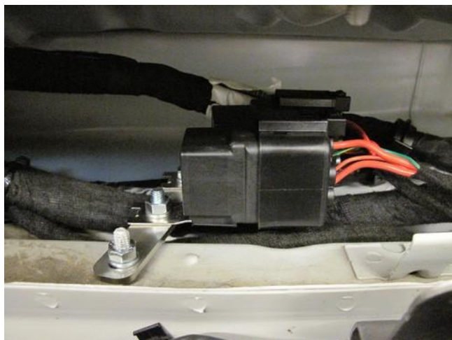
Mount bracket to wiper box.
