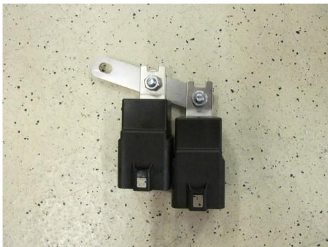
Mount relays to bracket with M6 bolts, nuts and washers.
