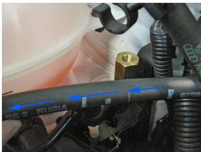
Mount just removed rubber ring to 8mm fuel hose. Cut hose on length.
