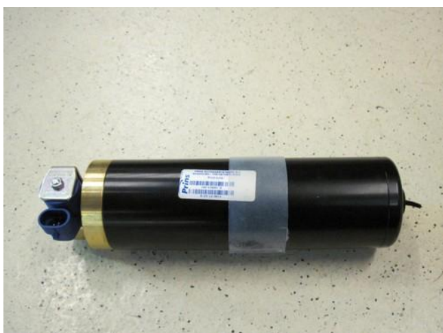
Put boost pump ring on boost pump. Mount boost pump in boost pump clamp (do not tighten clamp).
