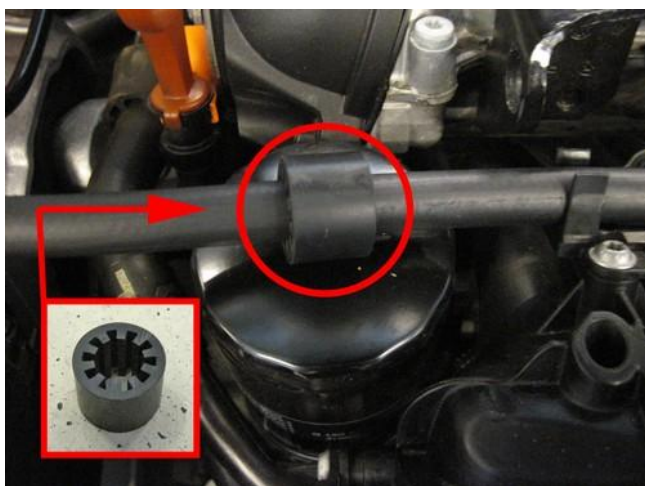
Mount just removed rubber ring to 8mm fuel hose. Cut hose on length.
