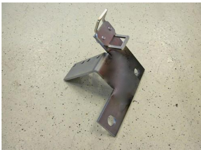
Mount boost pump clamp on bracket.
