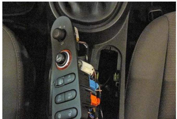
Mount switch. For easy connection / fitting remove panel.
