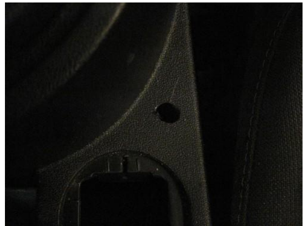
Mark hole for drilling. Drill hole Ø8.3mm
