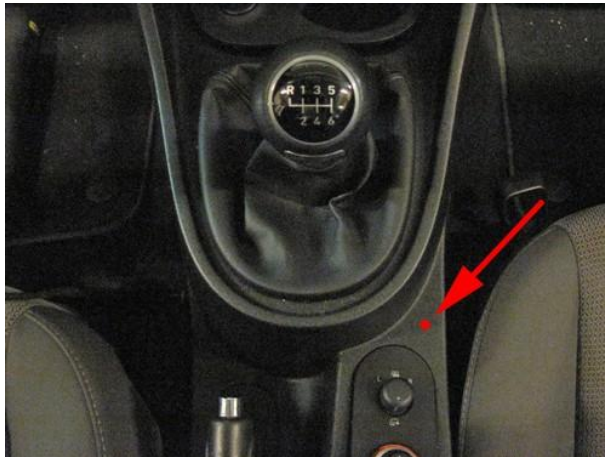
Mark hole for drilling. Drill hole Ø8.3mm
