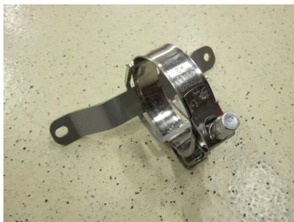
Mount bracket with boost pump clamp to original threaded ends.
