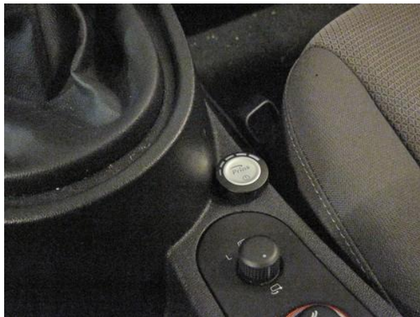
Mount switch. For easy connection / fitting remove panel.
