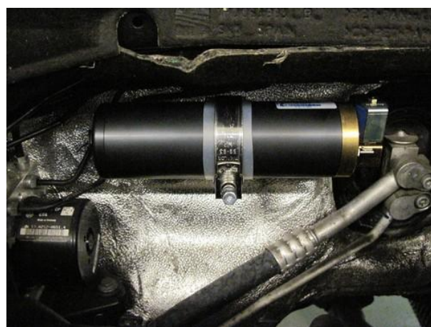
Mount boost pump with rubber ring to bracket/clamp.
