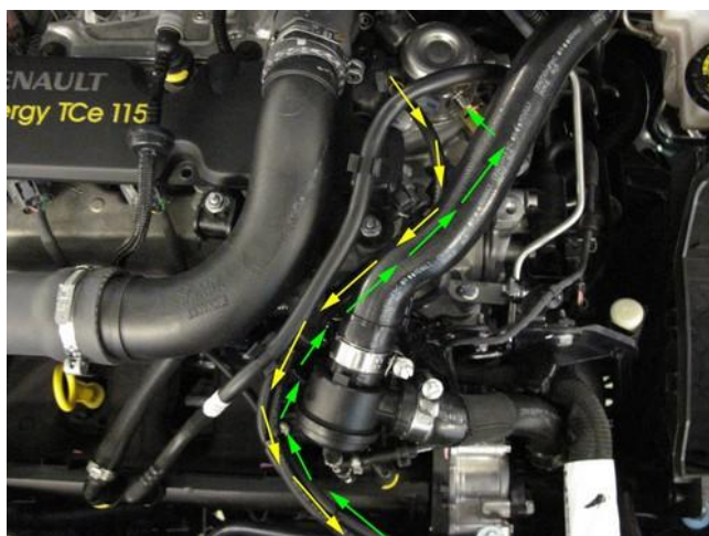
Mount hoses from FSU / FRU to HP pump.
