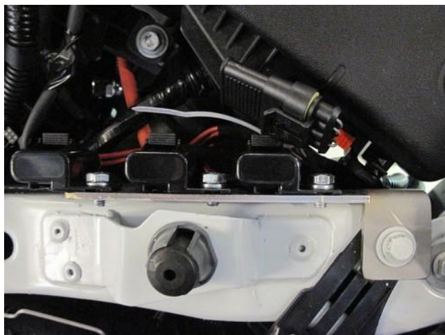
Mount fuse holders to bracket with M6 bolt & spring washer. Mount bracket to original bolt from left head light.
