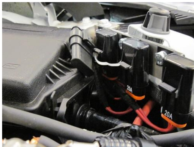
Mount fuse holders to bracket with M6 bolt & spring washer. Mount bracket to original bolt from left head light.
