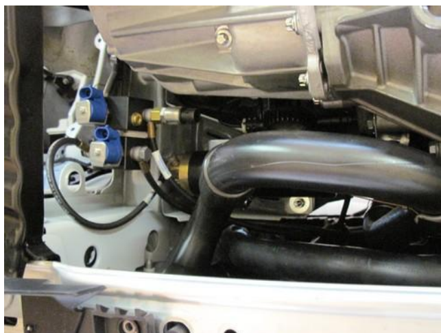
Mount hose from boost pump to FSU. Mount hoses from FSU / FRU to HP pump.
