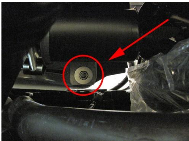
Mount bracket to vehicle below battery on 2 original bolts with big washers, spring washers and nuts.
