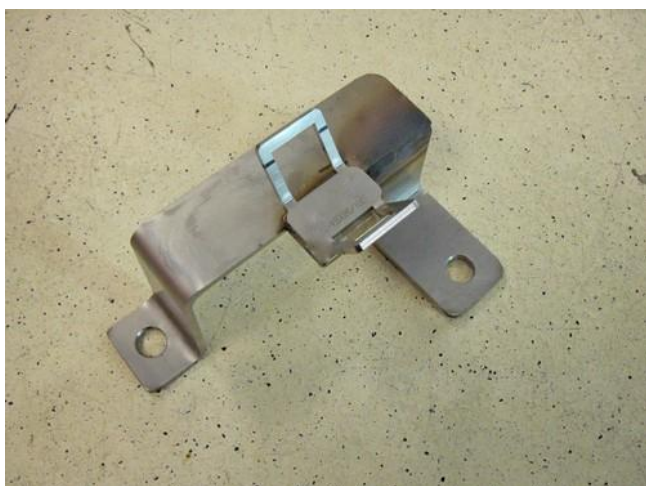
Mount boost pump clamp on bracket.
