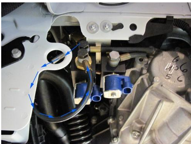
Mount hose from boost pump to FSU. Mount hoses from FSU / FRU to HP pump.
