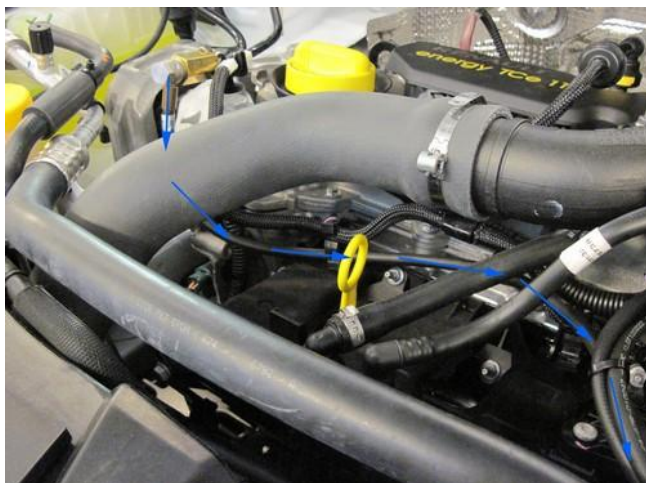
Mount fuel line (blue arrows) from adapter to the boost pump.
