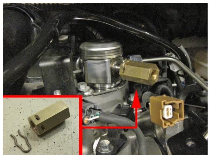
Mount hoses from FSU / FRU to HP pump. Mount adapter to HP pump.
