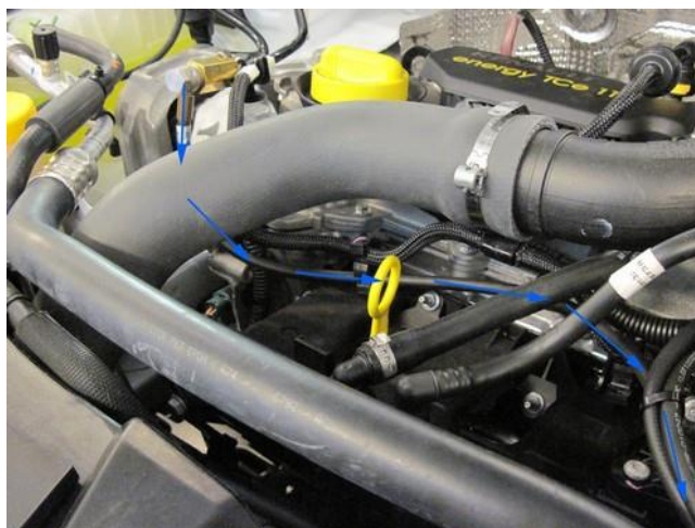
Mount adapter to original connection. Mount fuel line (blue arrows) from adapter to the boost pump.
