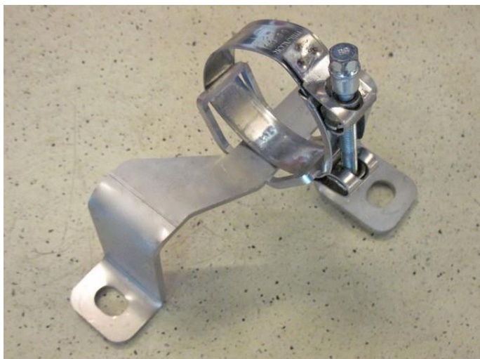
Mount boost pump clamp on bracket.
