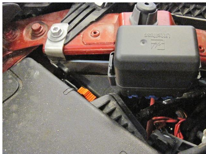
Mount bracket to original bolt from left head light. Mount the box on the bracket. Mount diagnostic connector to cap from box with a cable tie.
