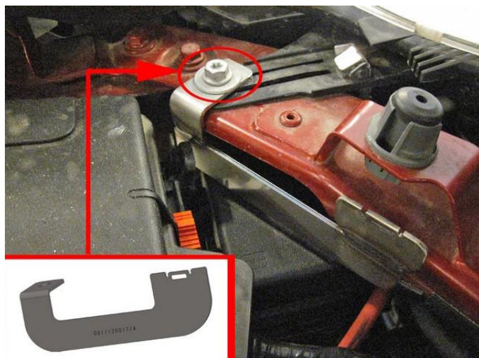
Mount bracket to original bolt from left head light. Mount the box on the bracket. Mount diagnostic connector to cap from box with a cable tie.
