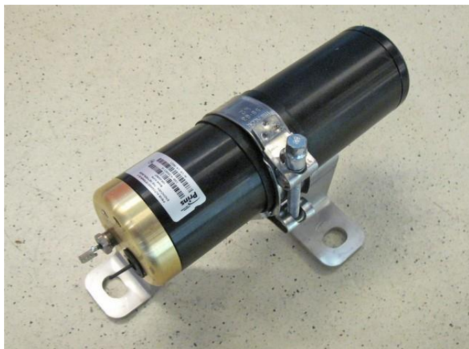
Mount boost pump in clamp with rubber ring in between. Mount bracket to vehicle below battery on 2 original bolts.
