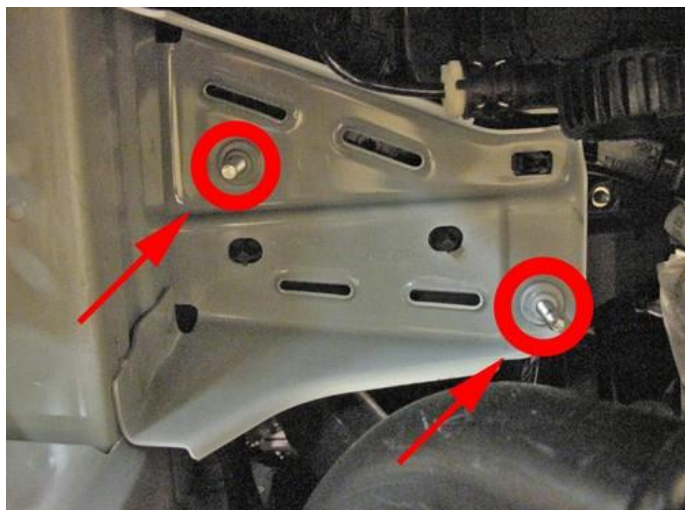
Mount boost pump in clamp with rubber ring in between. Mount bracket to vehicle below battery on 2 original bolts.
