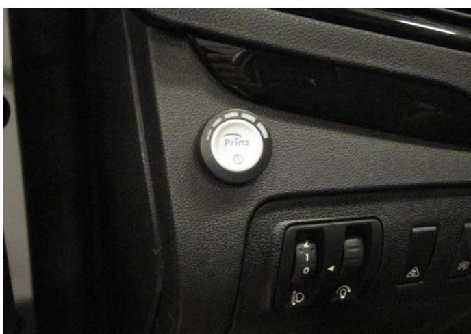
Drill hole 8,3mm for switch. Mount switch with supplied sticker.
