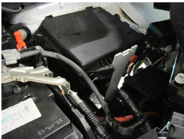
Mount the bracket to the original bolt. Mount the fuse/relay box.
