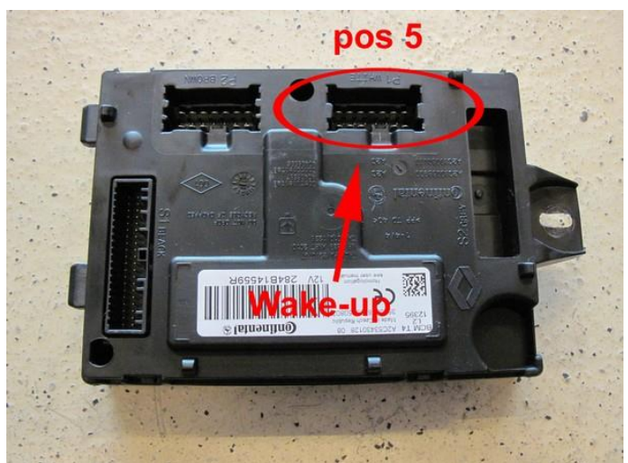
Body Control Module (for Wake-up connection).
