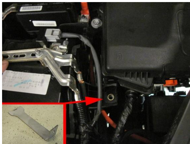
Mount the bracket to the original bolt.
