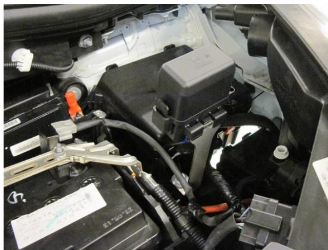
Mount the bracket to the original bolt. Mount the fuse/relay box.
