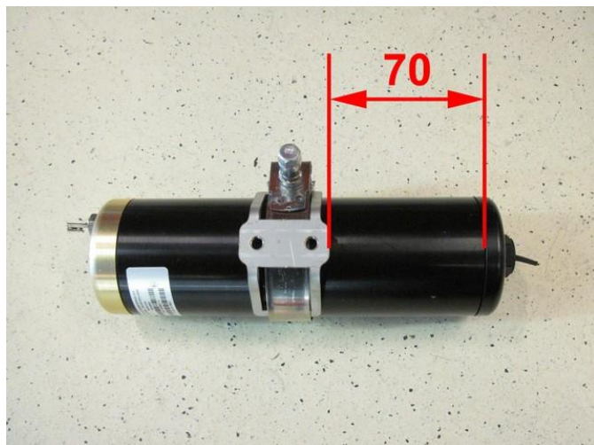
Mount boost pump with clamp & rubber to bracket.
