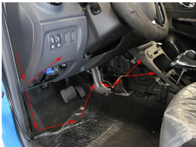
Wiring routing inside. Body Control Module (for Wake-up connection).
