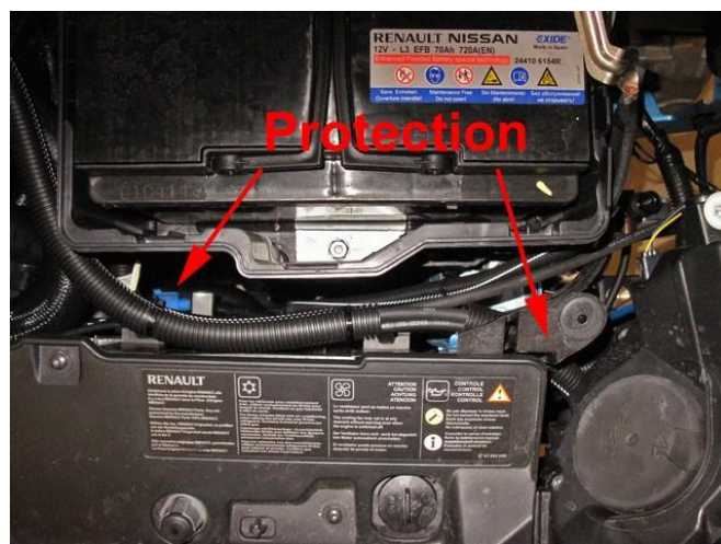
Hoses to FRU & FSU. Mount protection around hoses.
