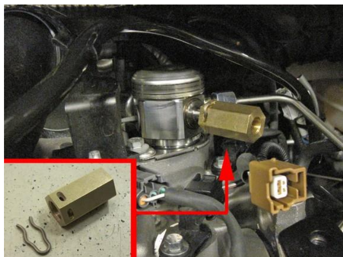
Boost pump -> FSU. Mount adapter to high pressure pump.
