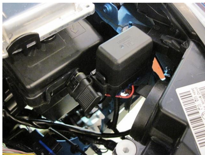
Mount the fuse-relay bracket to the original mounting bolt. Fuse-relay box with diagnostic connector.
