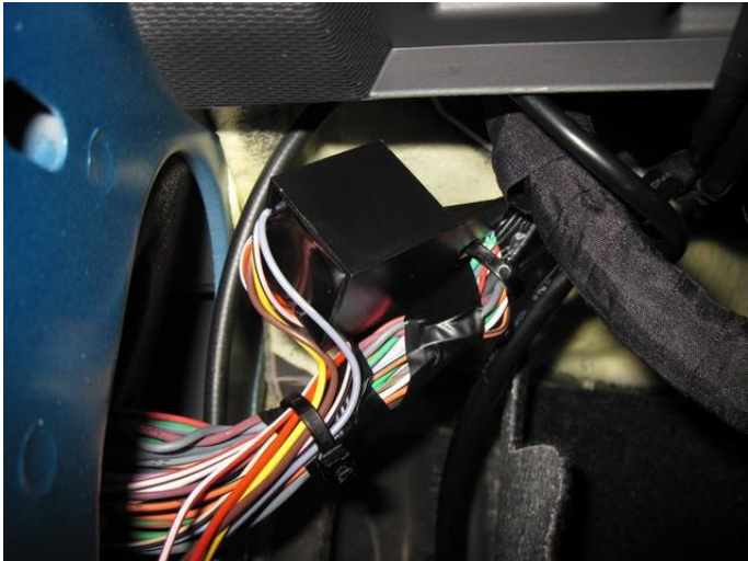
Mount fuel gauge reset module on the left side underneath the dashboard near the fuse box. Connection of the reset wires underneath left doorstep in wiring loom.
