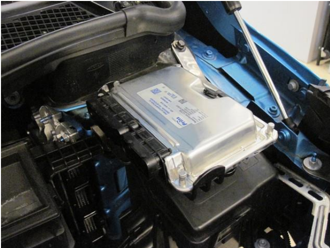
Mount the AFC. Mount the fuse-relay bracket to the original mounting bolt.
