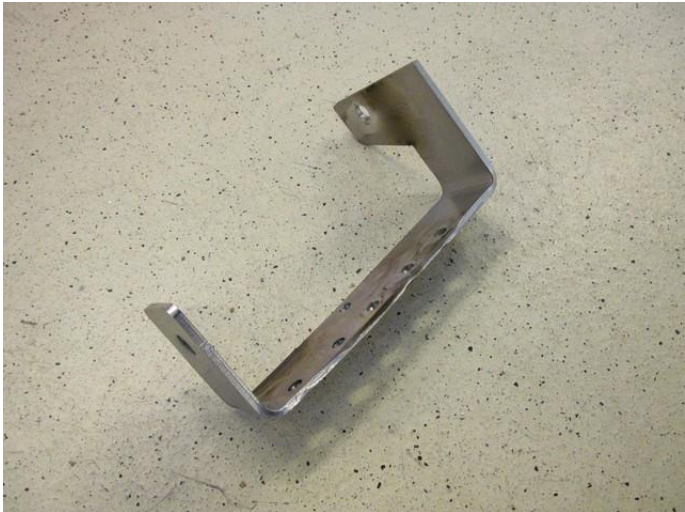
Mount Boost pump, FSU & FRU to bracket
