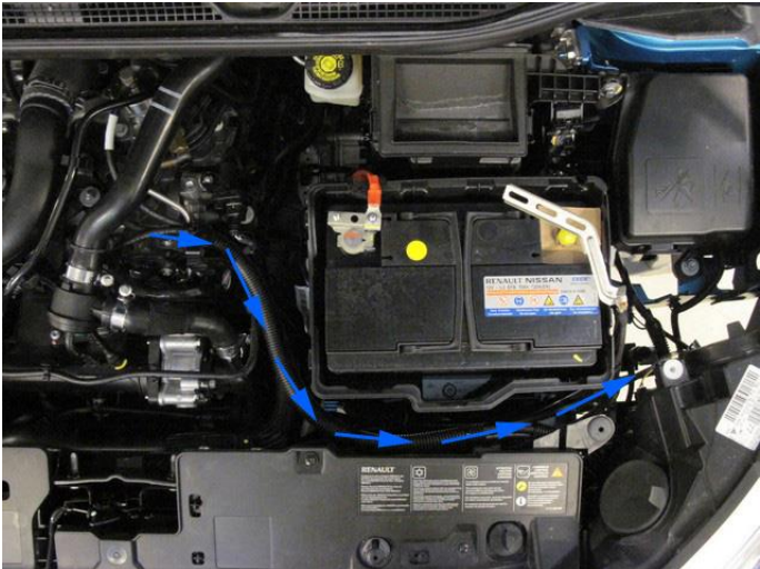
Remove original fuel line to HP pump. Mount adapter to original connection.
