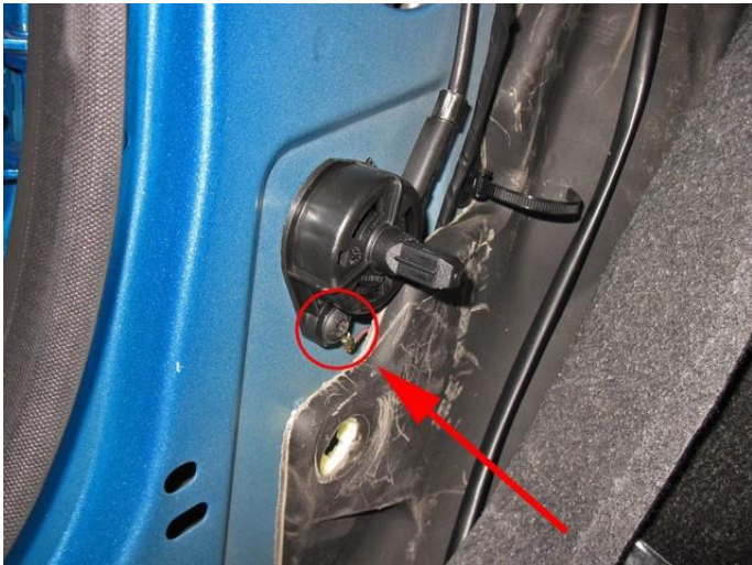
Ground of the reset module on bolt from hood latch.
