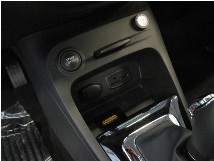
Drill hole Ø8,3mm. Mount switch.
