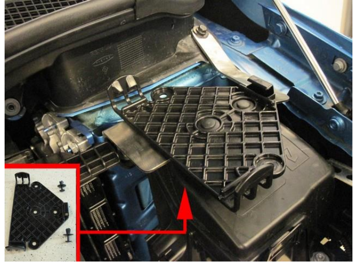
Mount the AFC bracket to the original bolts. Mount the plastic AFC clip.
