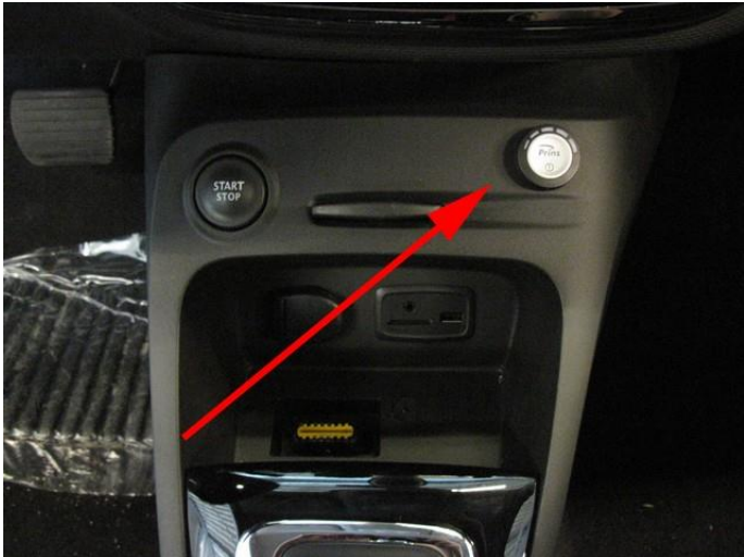
Drill hole Ø8,3mm. Mount switch.
