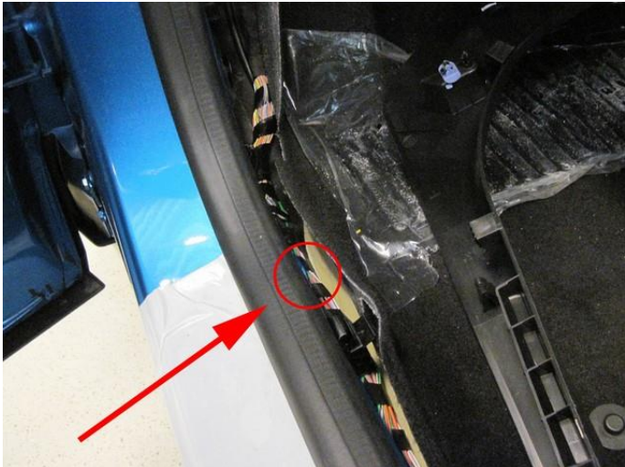
Mount fuel gauge reset module on the left side underneath the dashboard near the fuse box. Connection of the reset wires underneath left doorstep in wiring loom.
