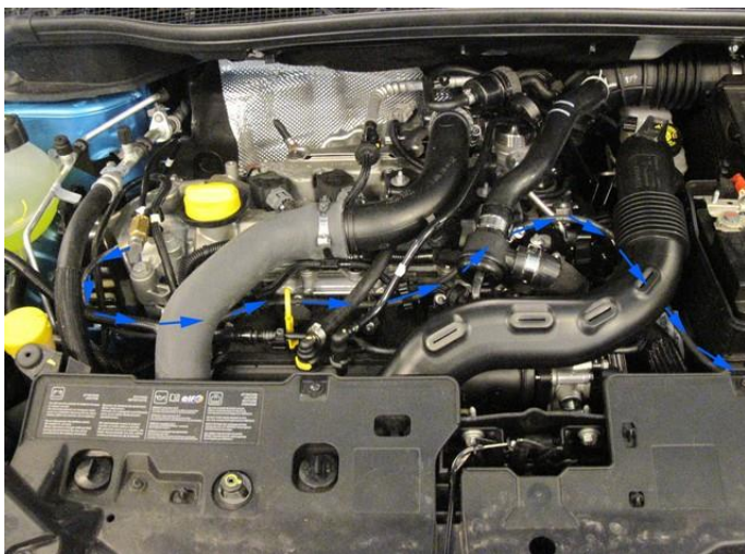
Remove original fuel line to HP pump. Mount adapter to original connection.
