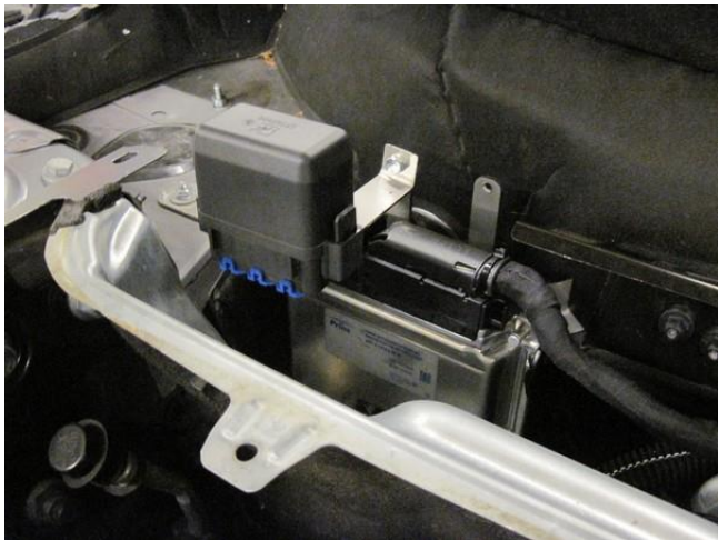
Mount fuse-relay bracket to AFC bracket. Mount fuse-relay box to bracket.
