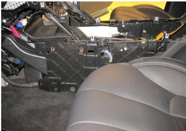
Remove pieces of the dashboard left & right. Remove left & right caps from center console.
