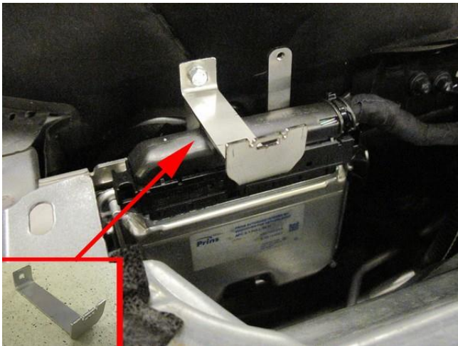
Mount fuse-relay bracket to AFC bracket. Mount fuse-relay box to bracket.
